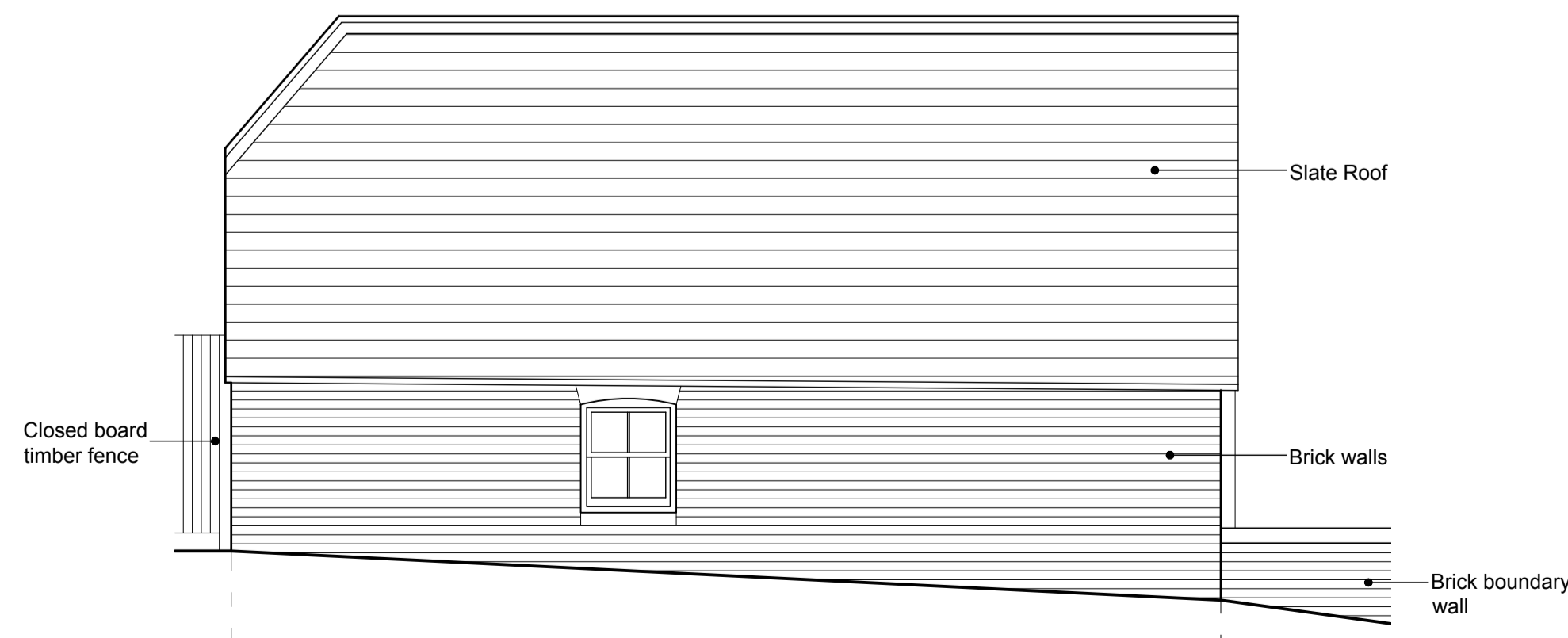
BRICK BUILDING - SIDE ELEVATION - SOUTH
